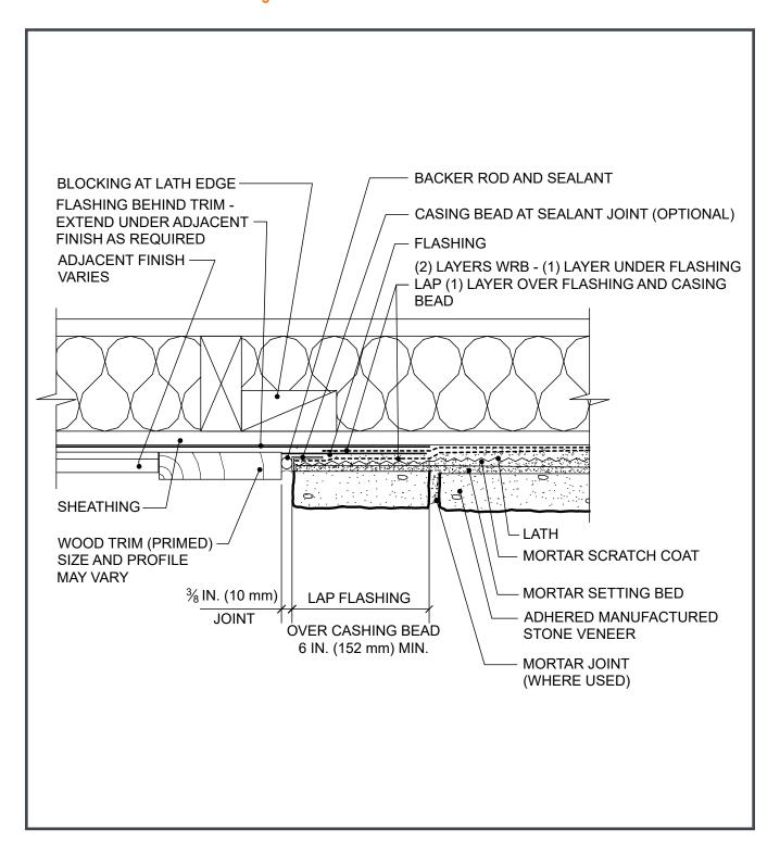
Figure 12b. Vertical Transition Over Continuous Insulation
