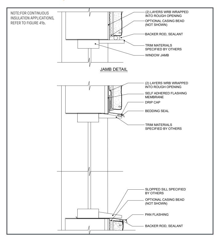
Figure 45. Wall-Section Multi-Floor Joint Detail
