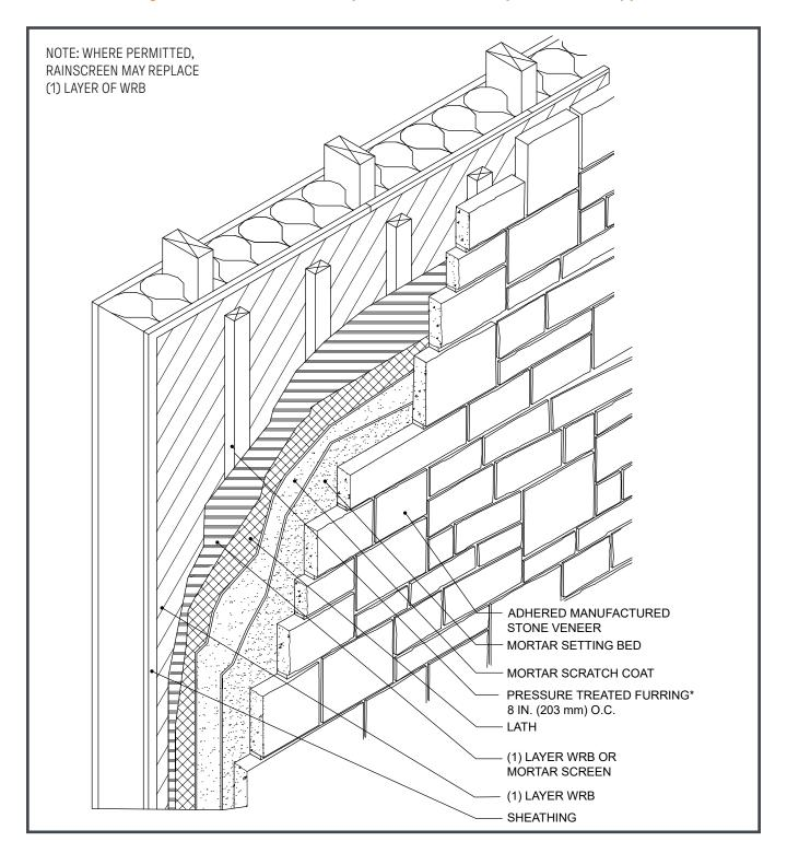
Figure 37. Foundation Wall Base - Rainscreen System
