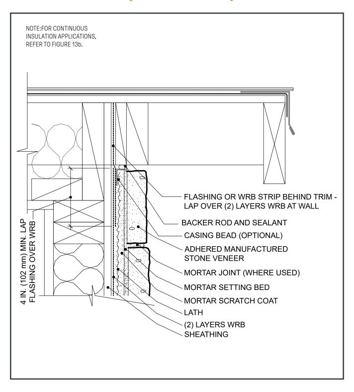
Figure 16. Rake - Flush
