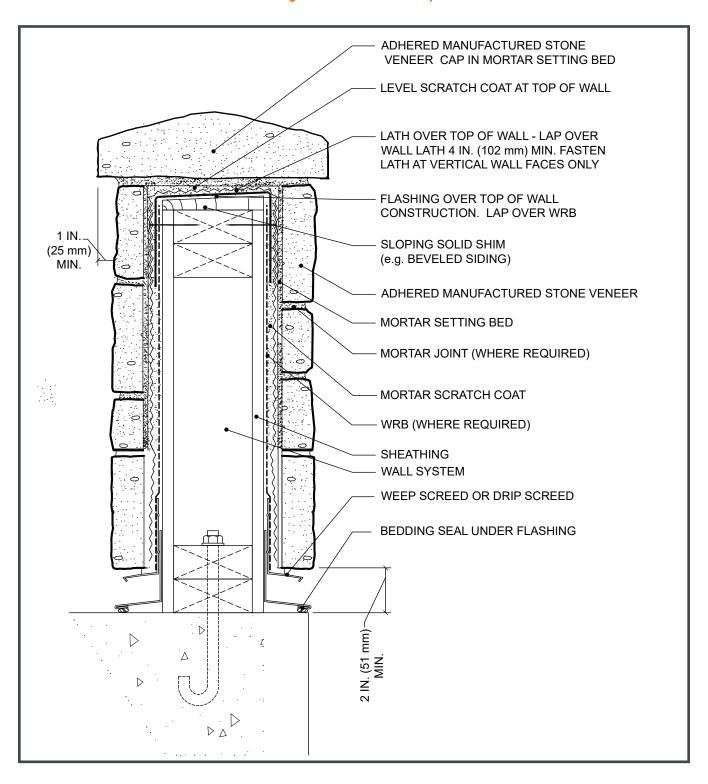
Figure 35. Wall Assembly - Rainscreen System - Membrane System
