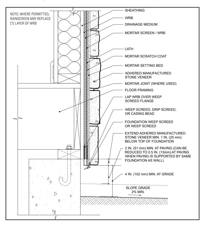
Figure 38. Typical Wall Section - Rainscreen System
