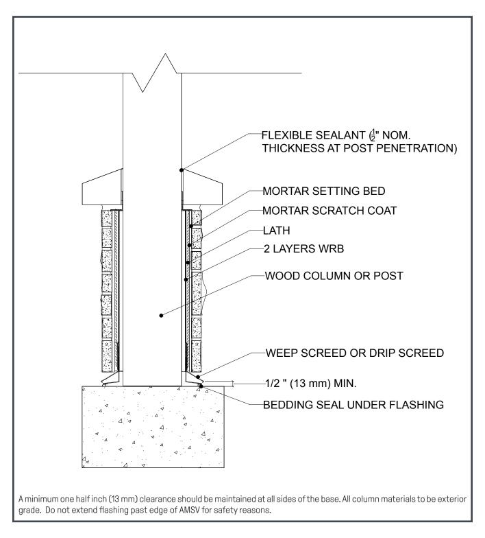
Figure 28. Penetration, Flanged
