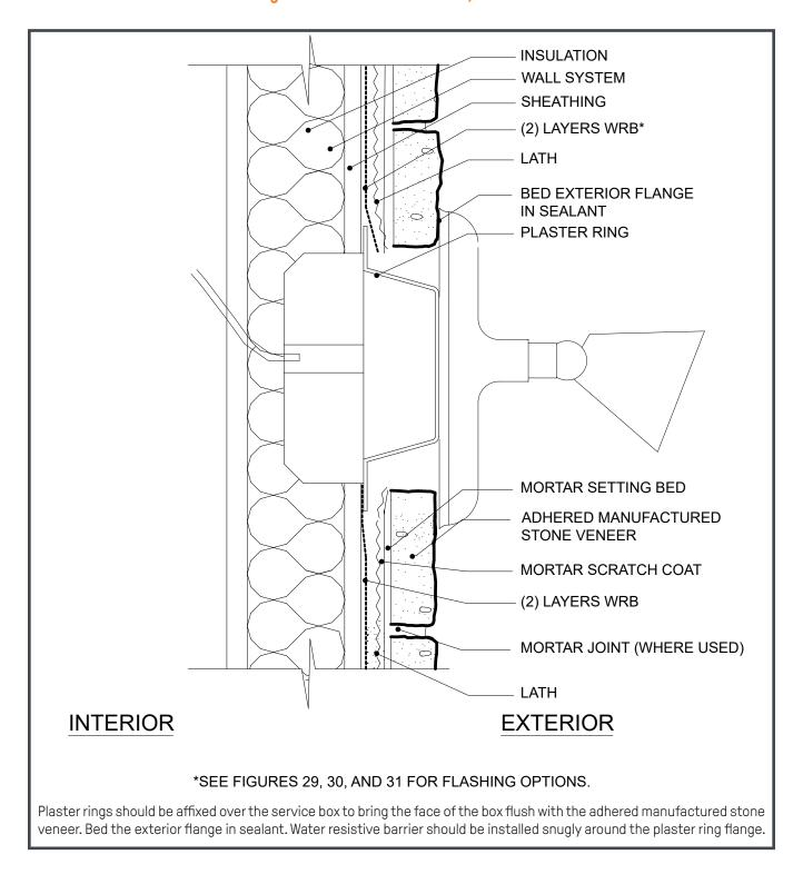
Figure 32. Penetration, Dryer Vent
