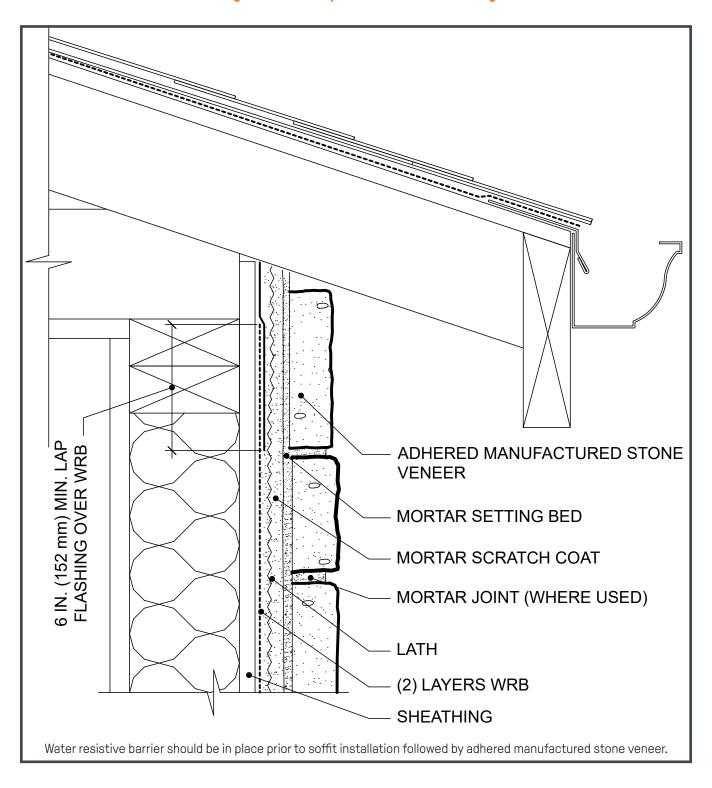
Figure 13b. Open Eave - Overhang Over Continuous Insulation
