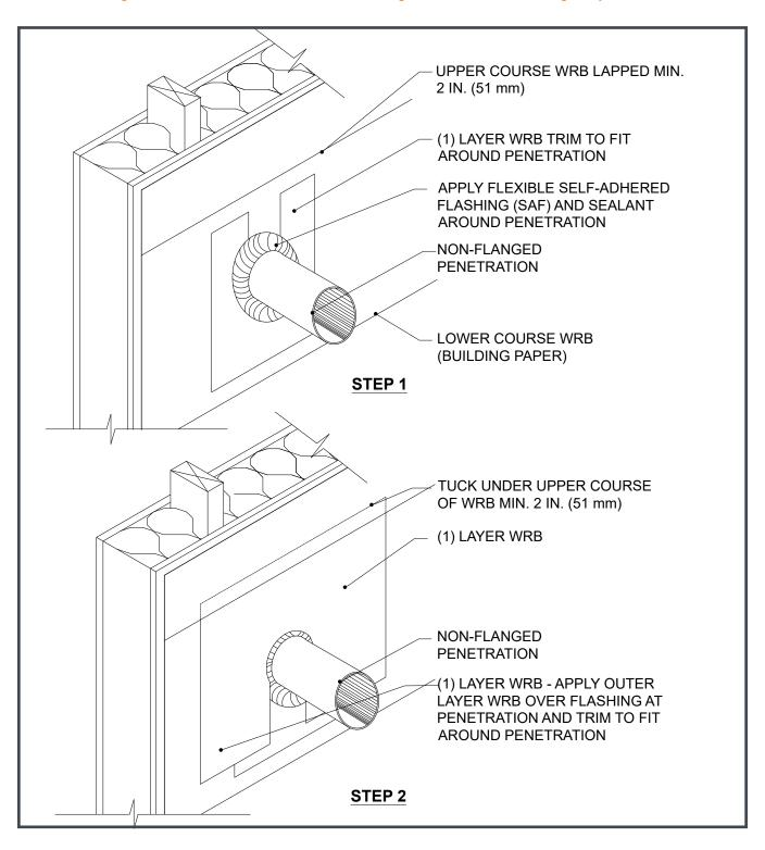
Figure 30. Penetration Non-Flanged, with Housewrap WRB
