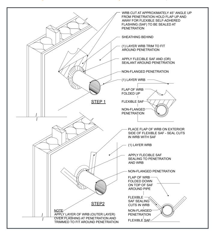
Figure 31. Penetration, Fixture
