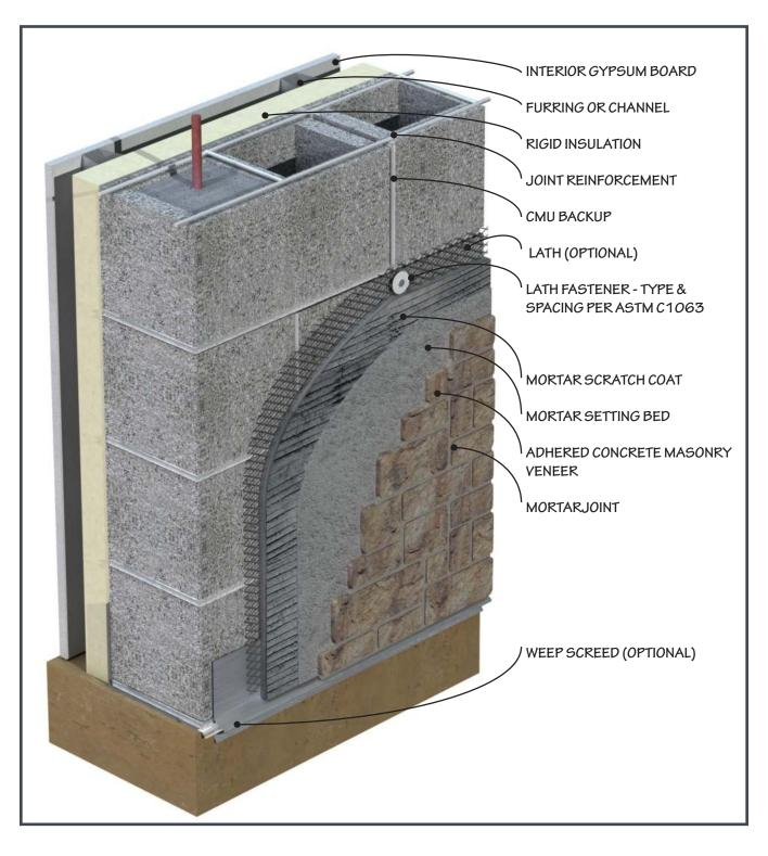
Figure 3. Wall Assembly Transition
