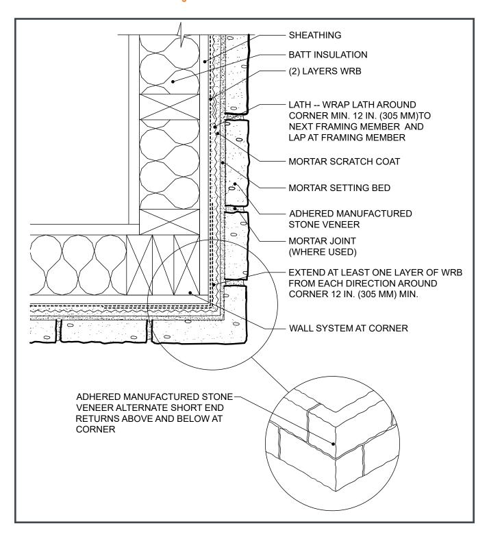
Figure 9b. Outside Corner Over Continuous Insulation
