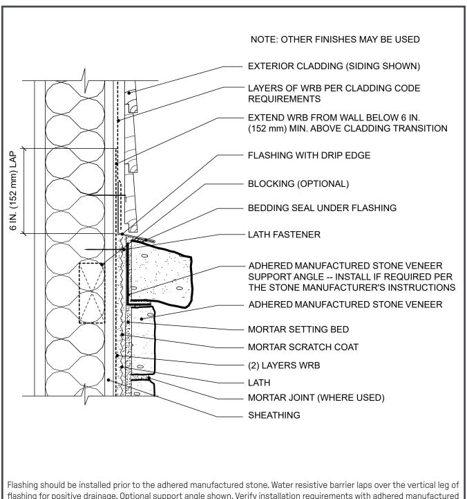
flashing for positive drainage. Optional support angle shown. Verify installation requirements with adhered manufactured stone veneer manufacturer.
