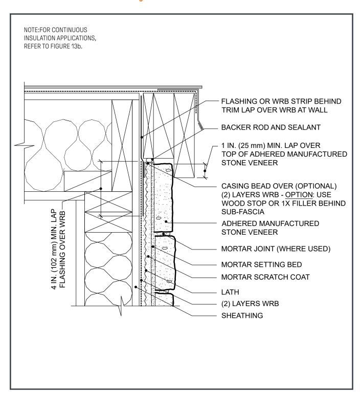
Figure 17a. Side Wall - Composition Shingles
