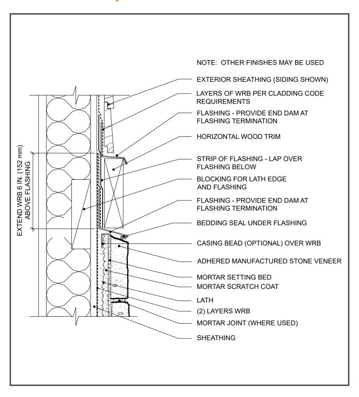
Figure 11b. Horizontal Transition Over Continuous Insulation
