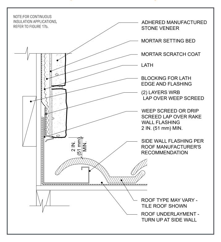
Figure 20. Side Wall - Tile Roofing Curbing
