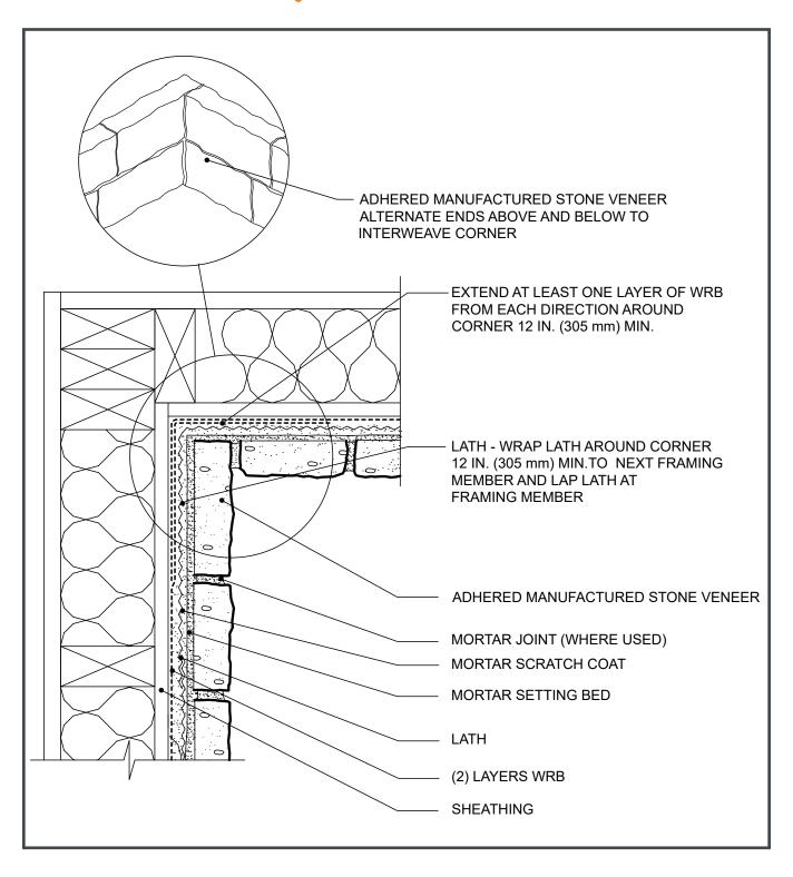
Figure 10b. Inside Corner Over Continuous Insulation
