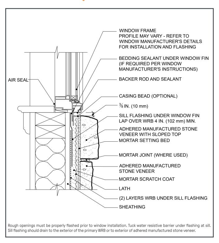
Figure 21b. Window Sill Over Continuous Insulation
