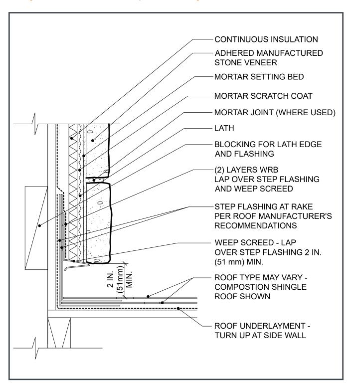
Figure 18. Side Wall - Composition Shingles Curbing
