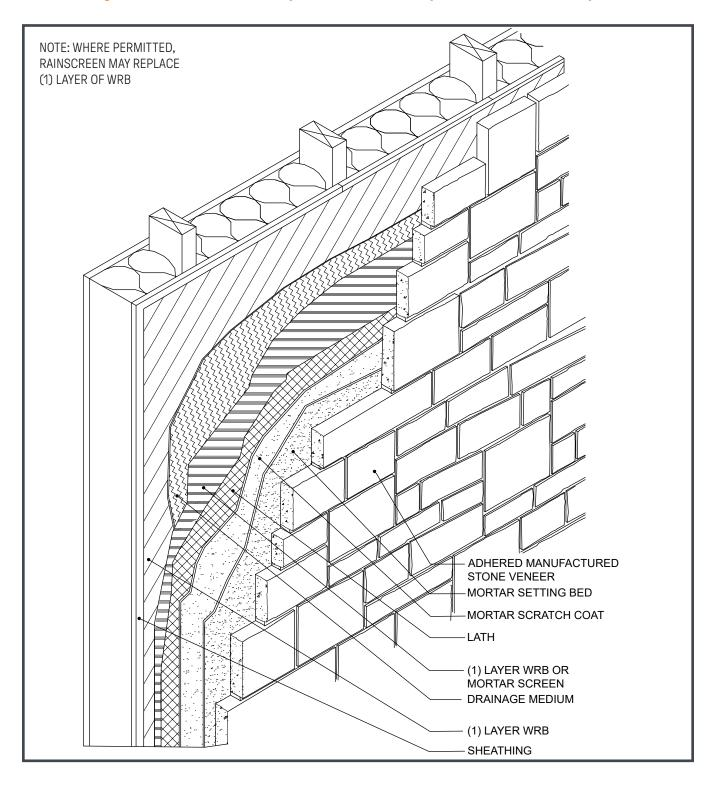
Figure 36. Wall Assembly - Rainscreen System - Strapped
