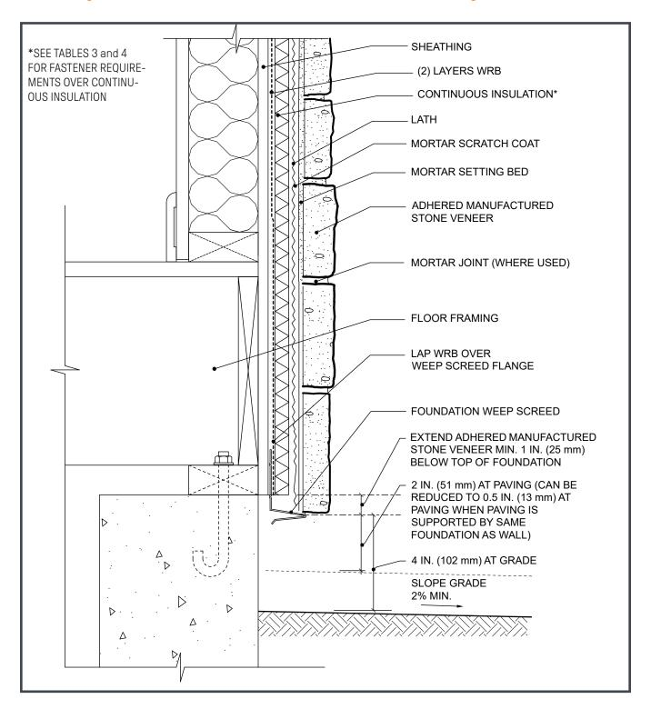
Figure 6. Foundation Wall Base - AMSV Overlapping Foundation
