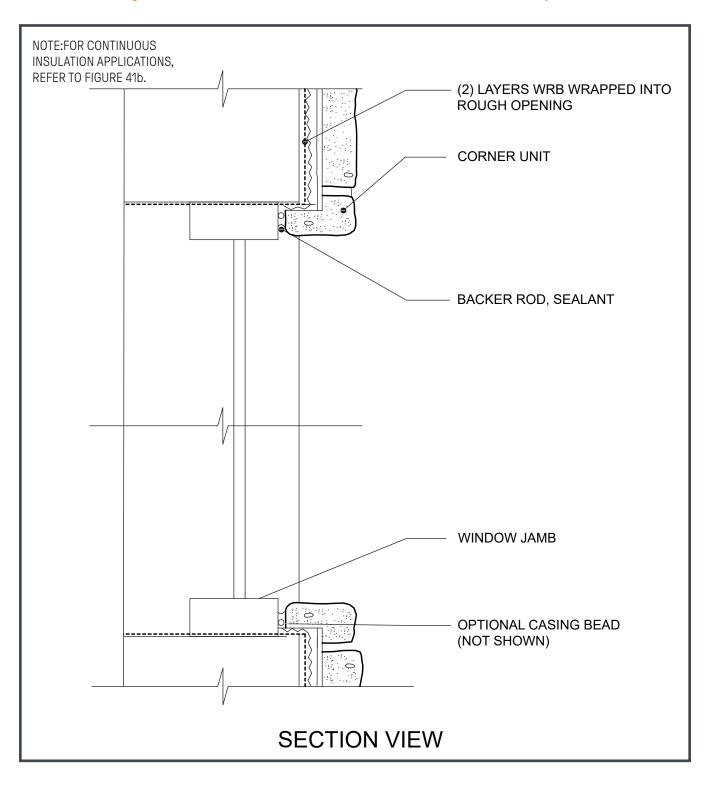
Figure 43. Commercial Storefront Window - Top View
