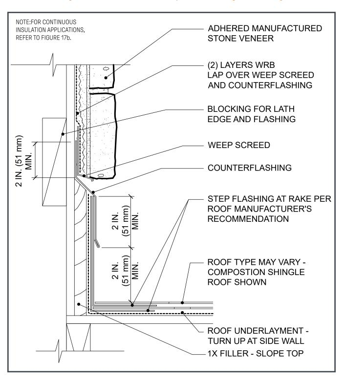
Figure 19. Side Wall - Tile Roofing
