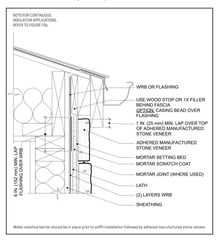
Figure 15. Rake - Overhang
